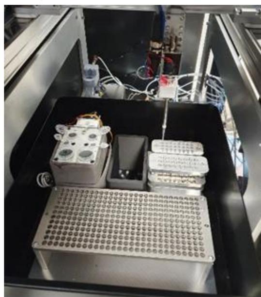
The air inlet and bespoke Impinger air sampler (left). The robotic arm and LAMP assay are placed in an enclosure (right).
