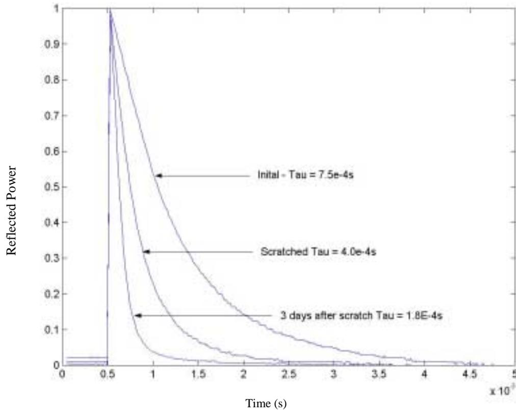
**Figure 7:** Reflected microwave intensity versus time illustrating introduction of surface damage and subsequent oxidation (sample temperature = 89K).
