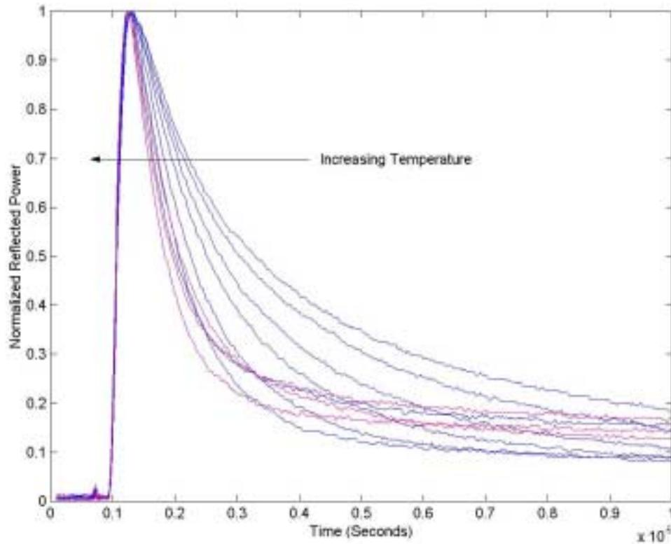
**Figure 4:** Reflected microwave power versus time from 250K to 89K for an as-cut CZT sample.
