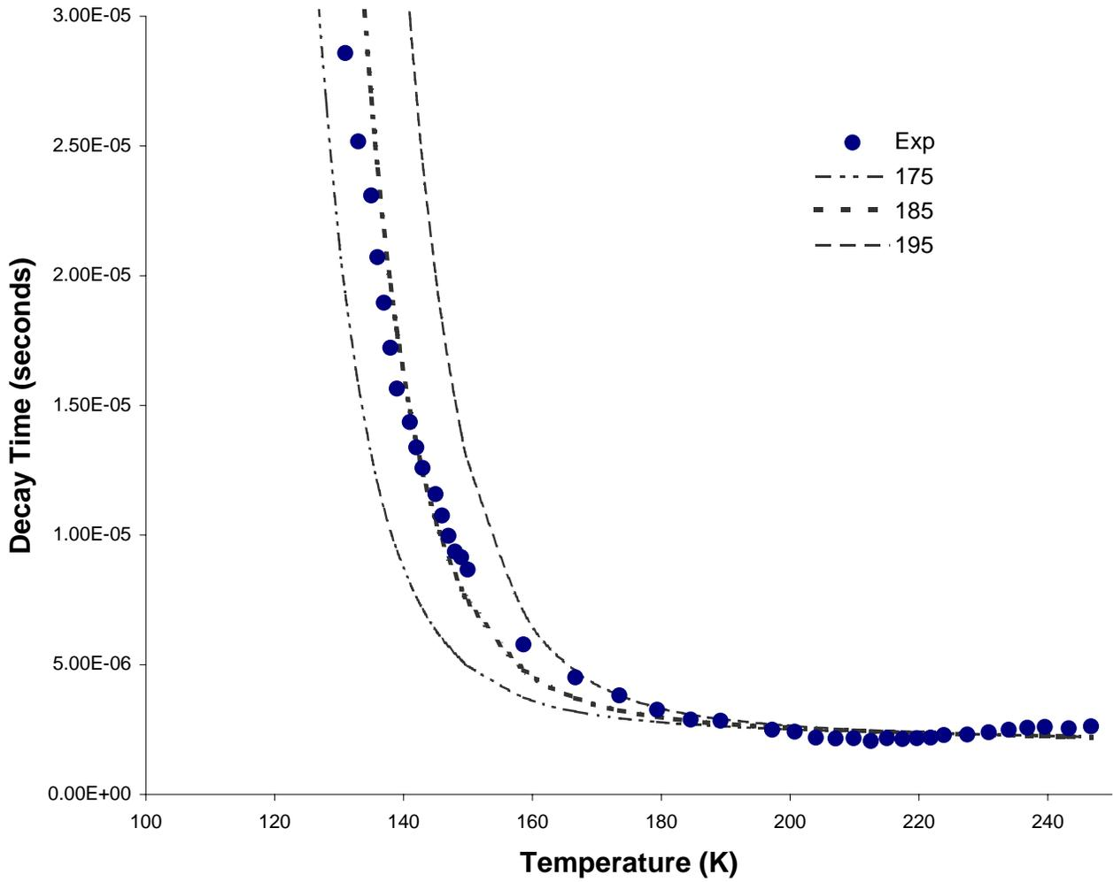
**Figure 3:** Plot of decay time versus temperature. The dots are the experimental data. The dashed lines are the results of a trapping model.
