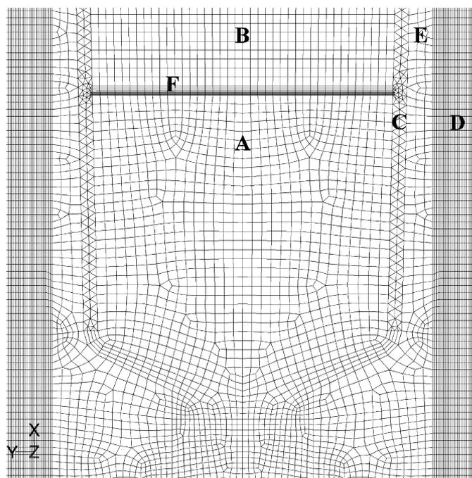
Fig. 1. Detailed view of 2D mesh section, illustrating melt (A), head vapor space (B), crucible (C), cylindrical graphite heaters, supports, and argon-filled vapor spaces (D), argon-filled internal space (E), and boundary layer at the melt–vapor interface (F).
