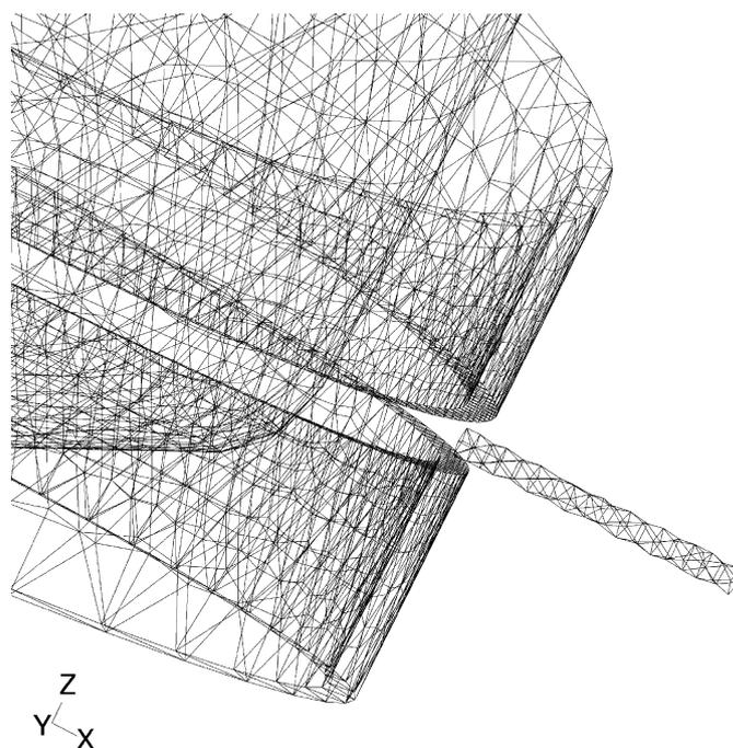
Fig. 2. Detailed view of 3D mesh segments, illustrating crucible, control thermocouple, and a heater section. Other furnace components have been rendered invisible in this view.
