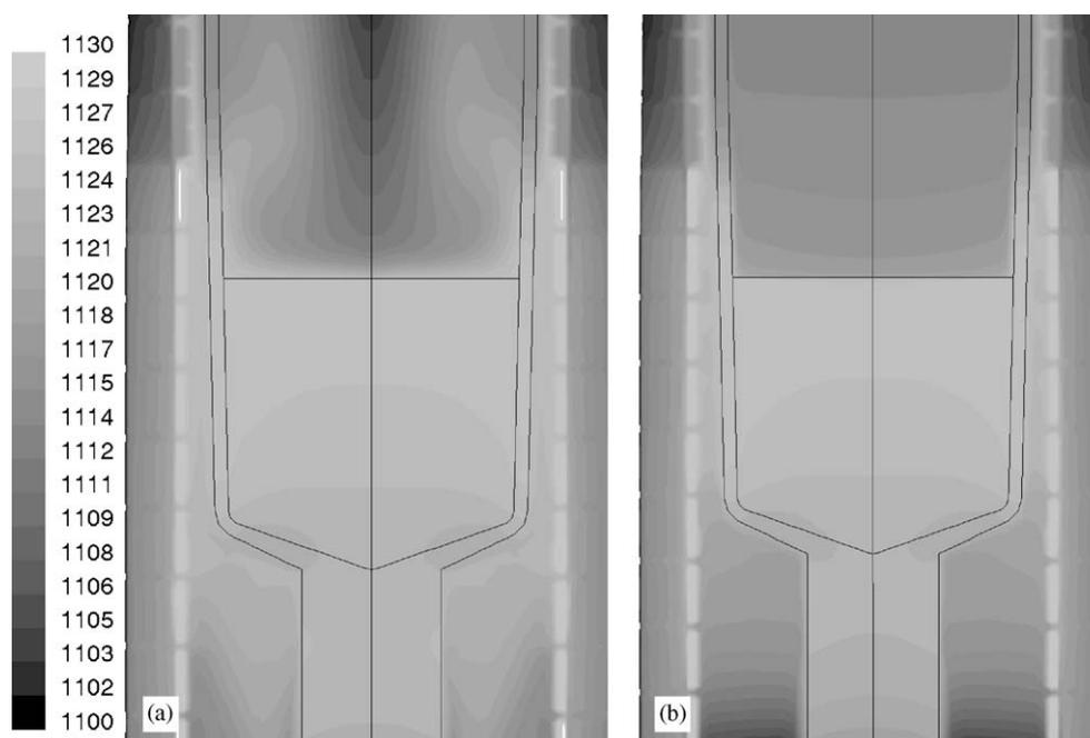
Fig. 9. (a) Temperature profile predicted by the laminar solver, for the lava insert. Top thermocouple temperature is 1108 °C, matching the experimental results. (b) Temperature profile predicted using the  $k-\epsilon$  turbulence model. Top thermocouple temperature is 1115 °C. Note that the temperature distribution in the lava insert is very similar in each case.
