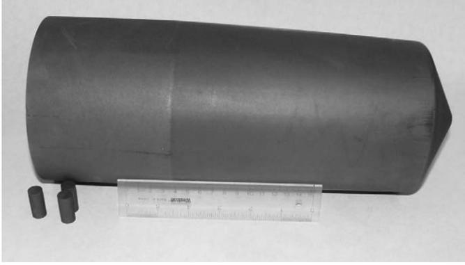
Fig. 3. Graphite insert. Graphite plugs, shown, were used to fill the thermocouple channel for non-centerline temperature measurements.
