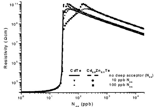
FIG. 2. Resistivity vs the concentration of deep donor at  $E_{d2} = E_v + 0.743 \pm 0.005$  eV is shown for CdTe and Cd-Zn-Te with 10% Zn, respectively. In addition to deep donor the presence of deep acceptors  $N_{da}$  at  $E_{d2} = E_v + 0.735 \pm 0.005$  eV was also considered (0, 10, and 100 ppb). When the Neumark conditions are satisfied, i.e., the concentration of deep donors exceeds the number of uncompensated acceptors the resistivity rises sharply.
