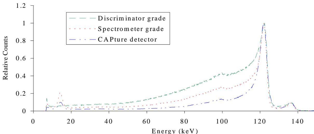
**Figure 3:** <sup>57</sup>Co response of CAPture™ technology and standard planar detectors
