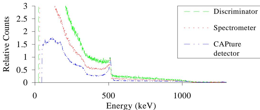
**Figure 5:** Response of CAPture™ technology and planar detectors to higher energy photons.
