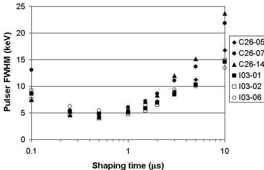
Figure 6. Pulser FWHM as a function of amplifier shaping time.
