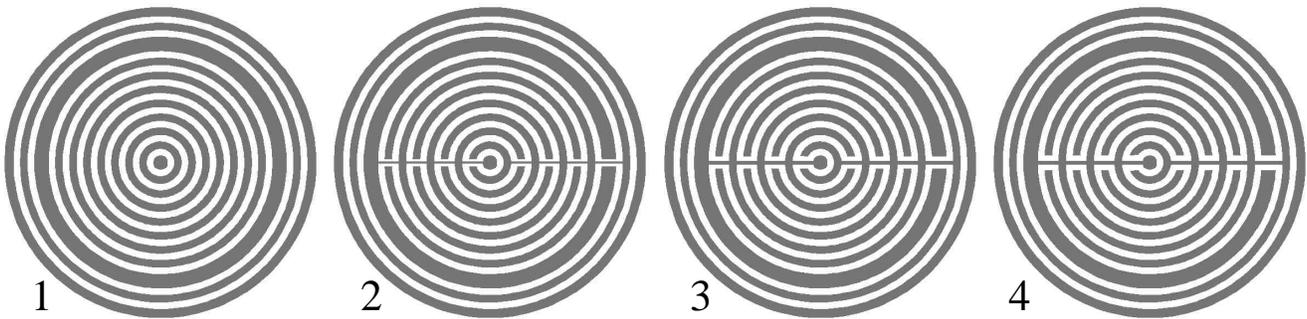
**Figure 4.** Grid patterns applied to cylindrical parts using photolithography: 1) No bus bar; 2) 50  $\mu\text{m}$  bus bar with 100  $\mu\text{m}$  gaps; 3) 100  $\mu\text{m}$  bus bar with 150  $\mu\text{m}$  gaps; 4) 100  $\mu\text{m}$  bus bar with 200  $\mu\text{m}$  gaps.
