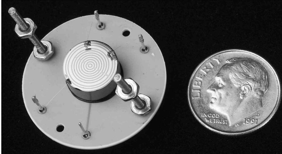
Figure 5. Detector I03-06 mounted on a ceramic substrate.
