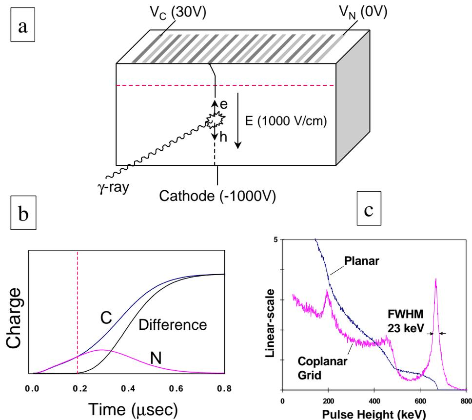
**Figure 1.** This illustration of coplanar grid technology includes the following: a) Coplanar grid detector geometry and nomenclature (C and N refer to the collecting and noncollecting coplanar grid electrodes, respectively). b) Charge pulse on the collecting, noncollecting, and difference electrodes. c) Comparison between pulse height spectra for the same device ( $10 \text{ mm} \times 10 \text{ mm} \times 5 \text{ mm}$ ) operated as a planar detector and as a coplanar grid detector.
