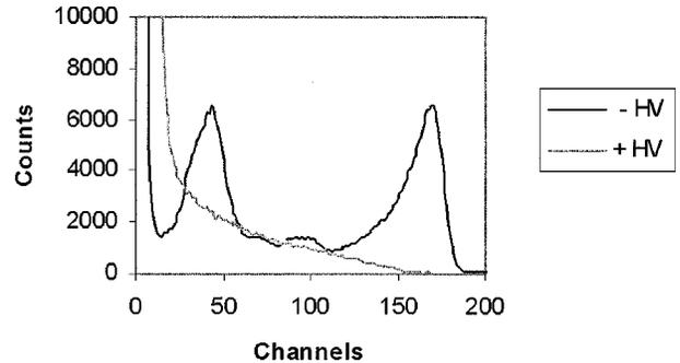
Fig. 3. Spectra comparison between hole-collecting mode ( $-HV$ ) and electron-collecting mode ( $+HV$ ) of the same CdZnTe detector where the  $^{241}\text{Am}$  source is placed at the frontside. The total charge ratio of hole-collecting mode and electron-collection mode is 2.66.
