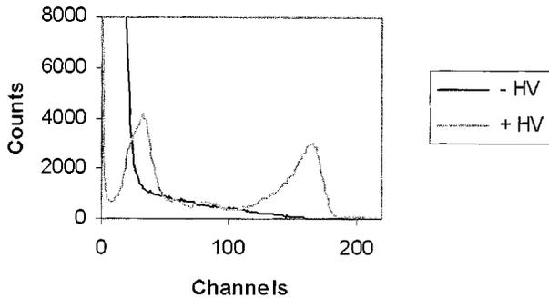
Fig. 2. Spectra comparison between hole-collecting mode ( $-HV$ ) and electron-collecting mode ( $+HV$ ) of a 0.5-mm-thick CdZnTe detector where the  $^{241}\text{Am}$  source is placed at the backside. The total charge ratio of hole-collecting mode and electron-collection mode is 0.66.
