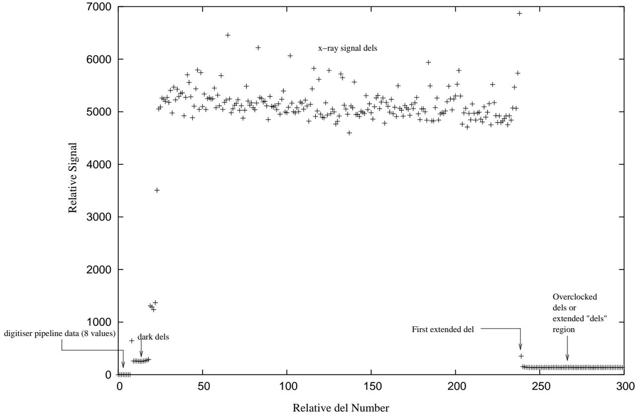
**Figure 3.** A plot of a detector readout line used in calculating the CTE. The plot is an average of several x-ray exposures. The large variation in response is due to the fixed pattern response (fpr) caused by intrinsic sensitivity variations of each del.
