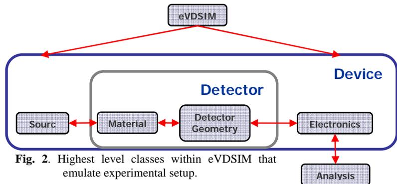
Fig. 2. Highest level classes within eVDSIM that emulate experimental setup.
