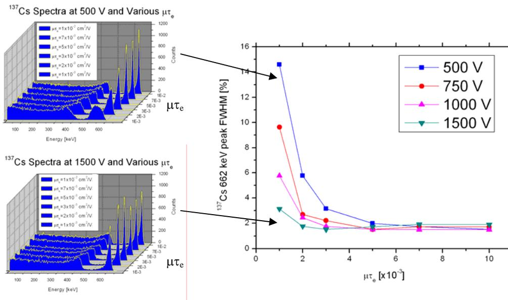
**Fig. 9.** Peak resolution (FWHM) at 662 keV for a  $10\times 10\times 5\text{ mm}^3$  CAPture™ Plus detector. Electron mobility-lifetime products are between  $1\times 10^{-3}\text{ cm}^2/\text{V}$  and  $1\times 10^{-2}\text{ cm}^2/\text{V}$ , and bias voltage is between 500 and 1500 volts. Spectra are shown at 500 V and 1500 V for all  $\mu\tau_e$ .
