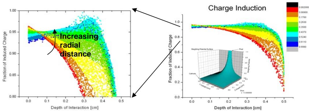
**Fig. 7.** (right) Charge induction map for a quasi-hemispherical detector. The x-axis is the depth of interaction measured in cm, and the y-axis is the fraction of charge that is induced. The inset is a mesh plot of the weighting potential. (left) A blow-up plot of the peak-forming region of the induction map. Increasing radial distance from the pixel center line is indicated by the arrow.
