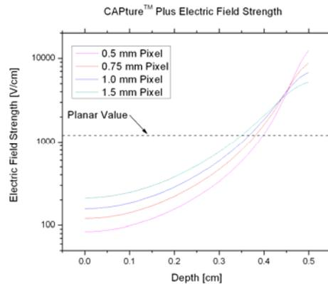
**Fig. 4.** (left) Mesh plot of the electric field strength within the 2D slice through the detector volume. The strength of the electric field within an equivalently biased planar detector is also shown as a uniform plane. (right) The field strength along the center line of the pixel due to various pixel sizes.
