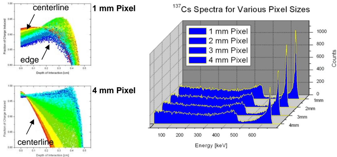
**Fig. 10.**  $^{137}\text{Cs}$  spectral performance for  $10\times 10\times 5\text{ mm}^3$  quasi-hemispherical designs with varying pixel size. The induction map on the top left is for a 1 mm pixel, while the induction map on the bottom left is for a 4 mm pixel.
