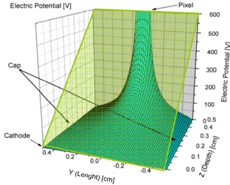
**Fig. 3.** (left) Quasi-hemispherical detector with 2D plane cut through the center of the pixel. (right) The electric potential [V] within the 2D plane is shown as a mesh plot. The electric potential of a planar detector at the same bias voltage is also shown.
