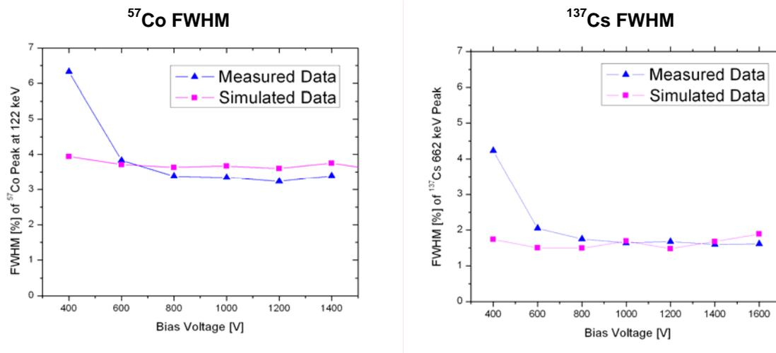
**Fig. 13.** Comparison of measured (triangles) and simulated (squares) FWHM peak resolutions for  $^{57}\text{Co}$  (left pane) and  $^{137}\text{Cs}$  (right pane) sources.
