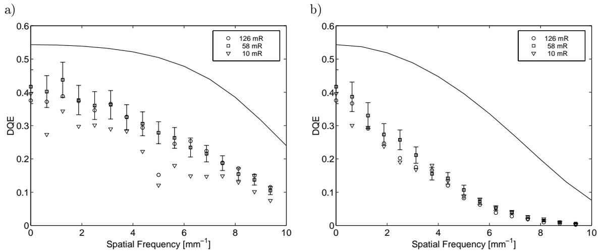
**Figure 7.** DQE in the slot (a) and scan (b) directions for detector #3. Experimental results at three detector exposures are shown, and the theoretical prediction based on the cascaded model presented in Section 3. Error bars are shown on a single curve for clarity.
