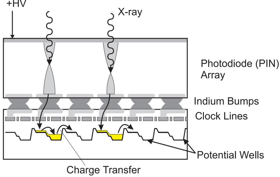
**Figure 1.** Cross section of the hybrid detector. Liberated charges produced by absorption of an x ray are swept to the electrodes on the PIN diode. Charge is transferred to the CCD by the indium bump bonds, and transferred down a column as a charge packet by controlling the clocking gates in the CCD.
