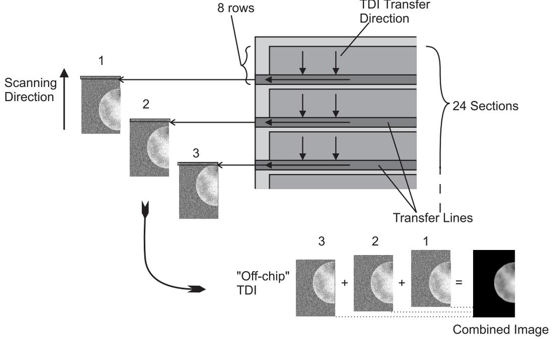
**Figure 2.** Schematic of the novel two-stage TDI process. The detector is divided into 24 sections, each of which performs normal TDI over 8 rows. The charge signal is transferred off-chip and integrated together with appropriate delays between each section. This figure is not to scale.
