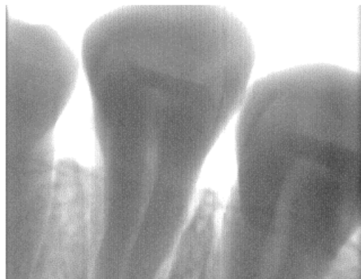
Figure 5: Image of a section of a jaw with teeth taken using a 1.5 mm thick hybrid silicon pixel detector.
