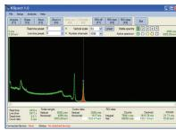
The cursor will change color to red and a "LLD" label will appear. Move the LLD as desired to cut out low-energy part of the spectrum or the noise peak. More details on the operation of K-Spect can be found under the 'Help' menu.
